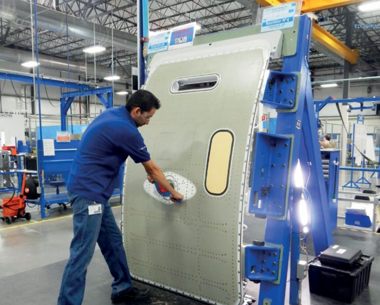
Image: Passenger Door mechanism check. Latecoere.
