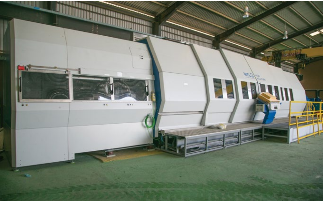
Image: Africa's first five-axis milling machine with a centre distance of 8m, courtesy of Thompson and Grace
