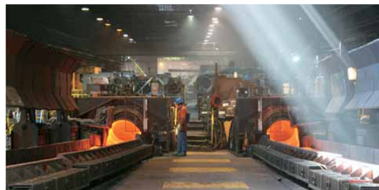
Ivaco bar coil laying heads at the start of the Stelmor-controlled cooling conveyors
