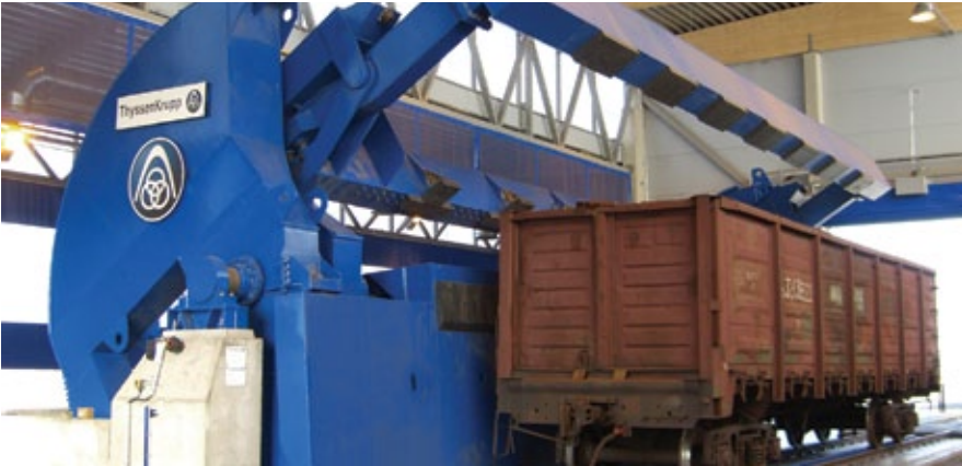
Side tipplers for unloading wagons with a simple clamping mechanism to discharge into a bunker alongside the tracks. Photo courtesy of ThyssenKrupp.
