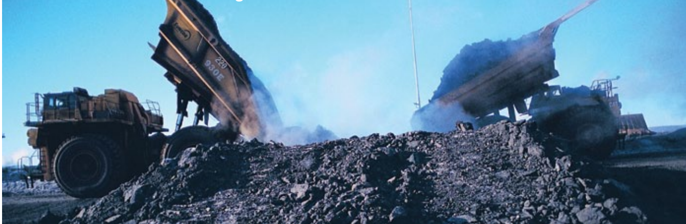
At the Suncor oil sands mine, huge 240 to 380 tonne trucks deliver about 500,000 tonnes of oil sand per day to the ore preparation plants. (Photo courtesy of Suncor Energy Ltd).
