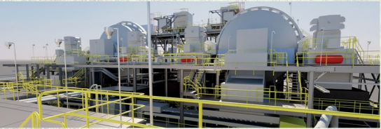
(Top and bottom) Digital twins of large-scale mine processing facilities delivered as a Revit model
