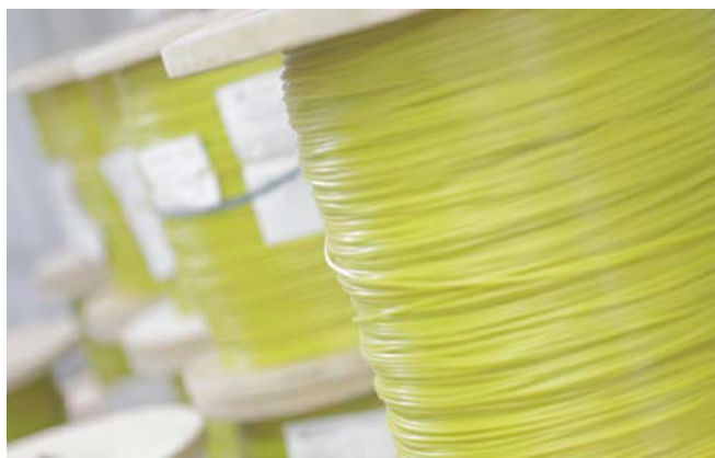
Detonating cord. Photo courtesy of Exsa.
